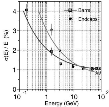
Fig. 1. ECAL energy resolution as a function of the electron energy.
