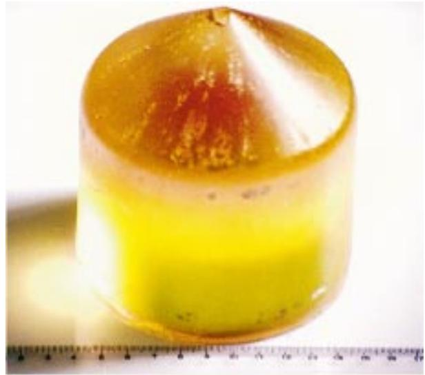
Fig. 4. A photo showing a sapphire boule grown at SIOM with diameter of 11 cm and length of 8 cm.
