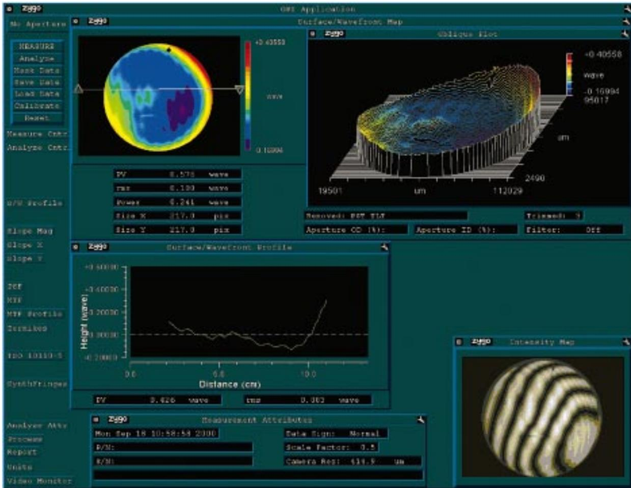
Fig. 8. Display of optical homogeneity measured by a ZYGO Mark-III interferometer at SIOM.
