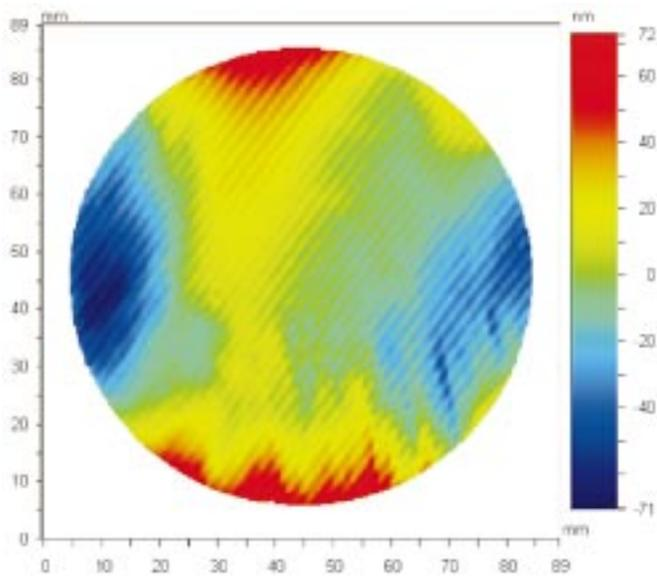
Fig. 9. A contour of optical homogeneity measured by a Wyko 6000 interferometer at Caltech.
