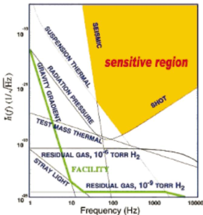
Fig. 2. The rms noise of LIGO I from various sources and corresponding sensitive region are shown as a function of frequency.
