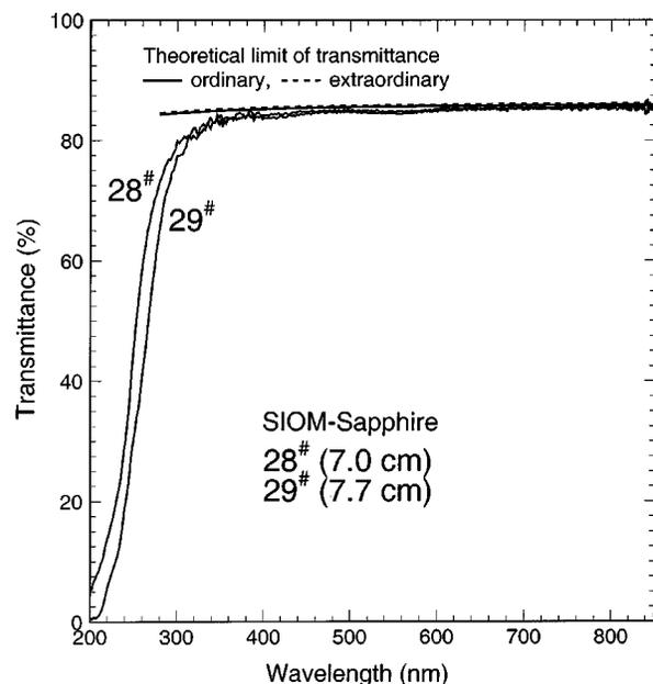
Fig. 7. Transmittance of SIOM samples #28 and #29 is shown as a function of wavelength and compared to the theoretical limit for light of ordinary and extra ordinary polarization.
