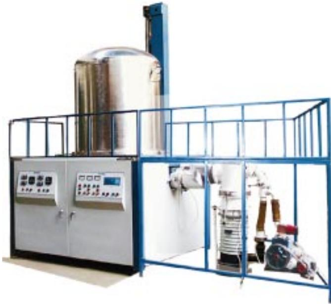
Fig. 3. A photo showing a TGT furnace used to grow sapphire crystals in SIOM.
