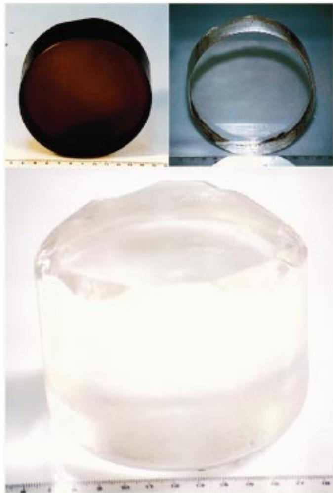
Fig. 6. Photos showing a sapphire sample after annealing in air (top left) and in H<sub>2</sub> (top right) and a full size sapphire sample after two-step annealing (bottom).
