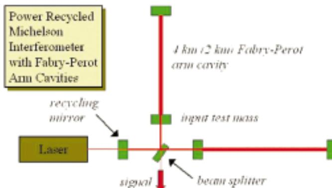
Fig. 1. A schematic showing the configuration of LIGO interferometer.
