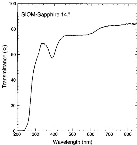
Fig. 5. Longitudinal transmittance spectrum is shown as a function of wavelength for a typical as-grown sapphire sample at SIOM.
