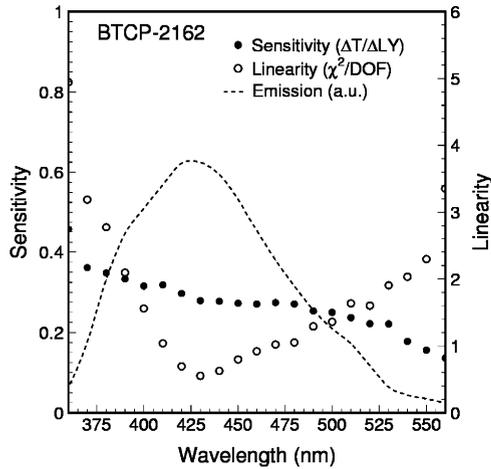
Fig. 6. Monitoring linearity and sensitivity are shown as function of wavelength for a sample [10].
