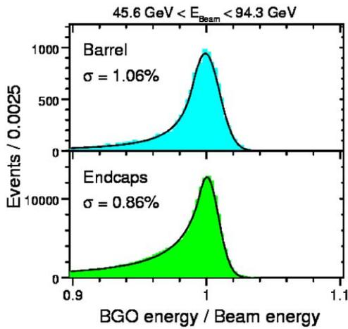
Fig. 4. Normalized Bhabha electron energy spectra measured by L3 BGO crystal calorimeter at LEP by using RFQ calibration.
