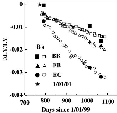
Fig. 1. Degradation of light output of the *BABAR* CsI(Tl) calorimeter in barrels (BB, FB) and endcap (EC) [2].
