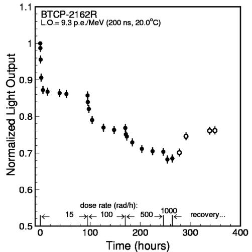
Fig. 5. Normalized light output of a PWO sample is shown as function of time during irradiation and recovery.
