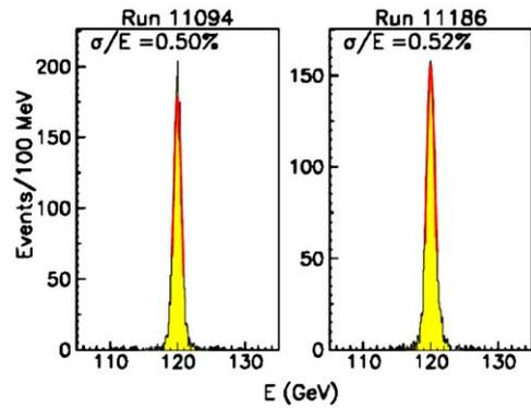
Fig. 8. Reconstructed energy spectra measured by PWO crystals before (left) and after (right) irradiation [11].
