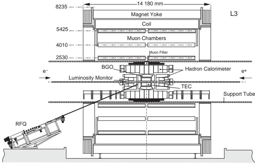
Fig. 3. Installation of the RFQ calibration system in the L3 detector at LEP [7].
