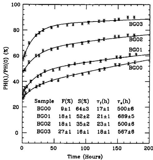
Fig. 2. Recovery of normalized light output is shown as a function of time after 2.5 krad irradiations for four BGO samples doped with different levels of Eu [5].
