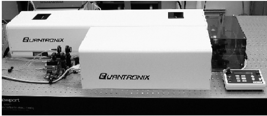
Fig. 6. (Back) Photo of the Quantronix laser system showing the Nd:YLF pump laser and (front) the tunable Ti:S laser.
