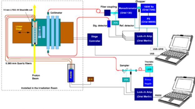
Fig. 2 A schematic showing the setup used to measure crystal's longitudinal transmittance *in situ* at LANL.
