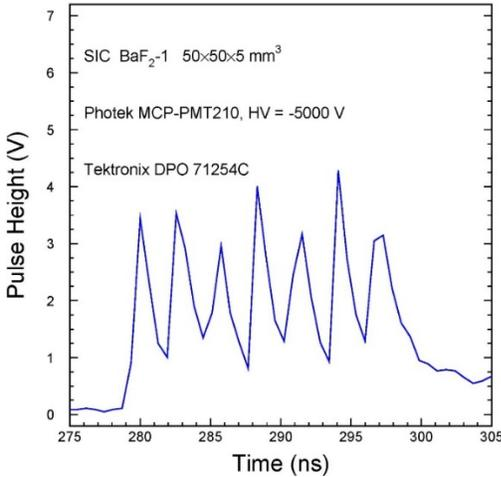
Fig. 4. Septuplet with 2.83 ns bunch spacing observed by BaF<sub>2</sub> coupled to the Photech MCP-PMT 210.
