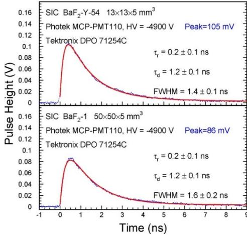
Fig. 3. Singlet bunch measured by BaF<sub>2</sub>:Y (top) and BaF<sub>2</sub> (bottom) coupled to the Photech MCP-PMT110.
