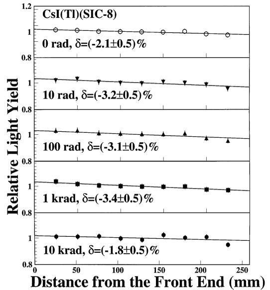
Fig. 5. The light response uniformities are shown as a function of integrated dose for a full size Csl(Tl) sample.
