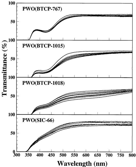
Fig. 2. Longitudinal transmittance of PbWO<sub>4</sub> samples, showing radiation-induced absorption bands.
