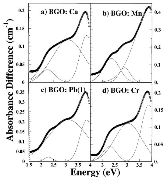
Fig. 15. Radiation-induced absorption spectra of four doped BGO samples (1 × 3 × 1 cm) are decomposed into three common absorption bands.
