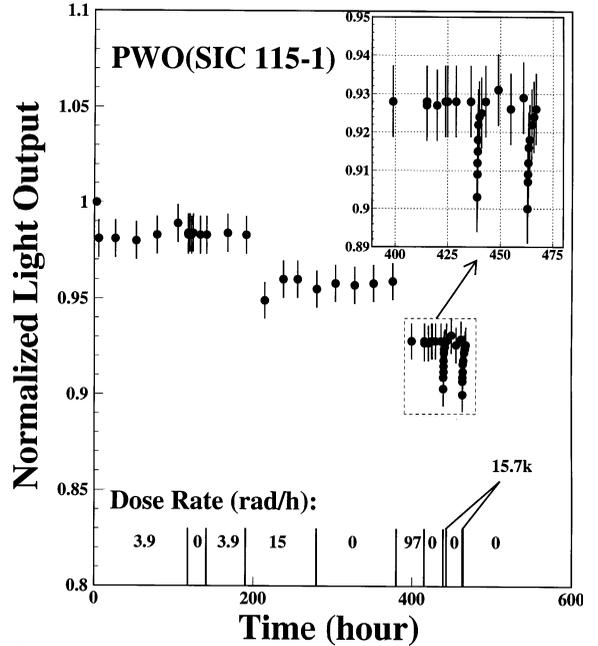
Fig. 10. The dose rate dependence is shown for a 5 cm  $\text{PbWO}_4$  sample SIC 115-1.
