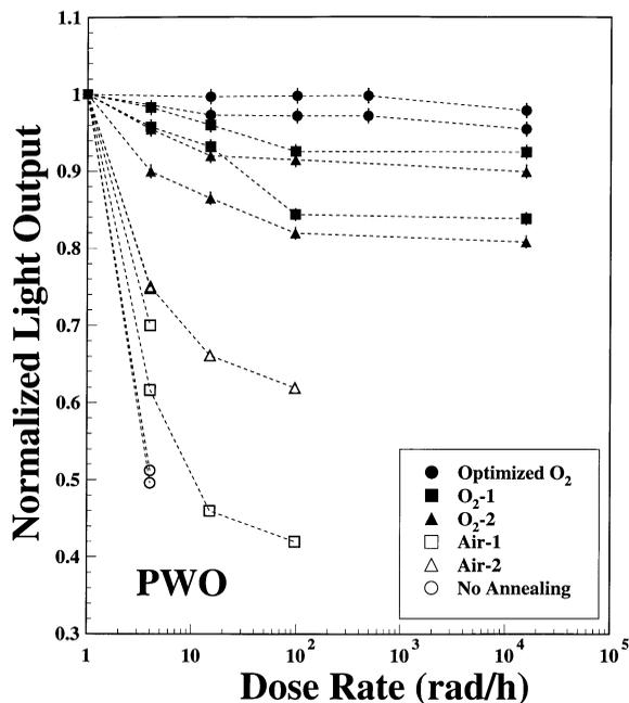
Fig. 16. Normalized light output at the equilibrium is shown as a function of the dose rate for six pairs of small ( $2 \times 5 \times 2$  cm)  $\text{PbWO}_4$  samples treated with different post-growing thermal annealing conditions.
