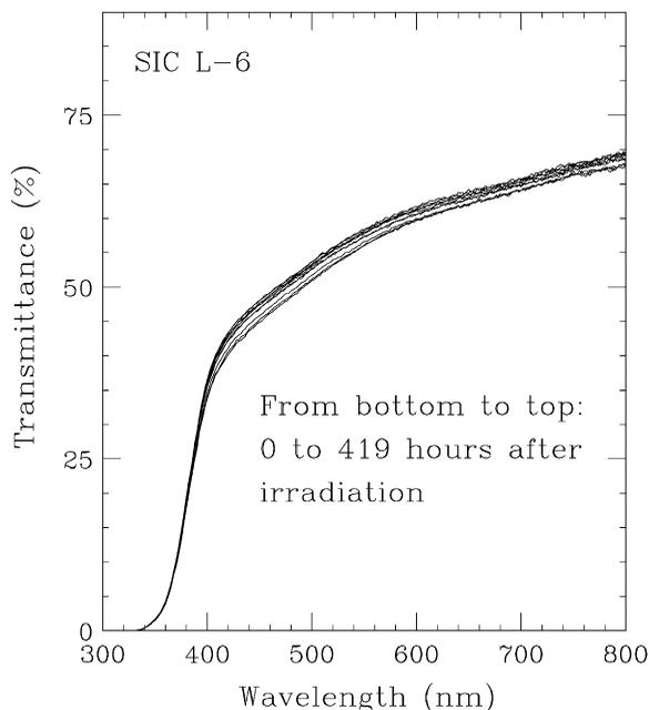
Fig. 5. Transmittance recovery at room temperature.
