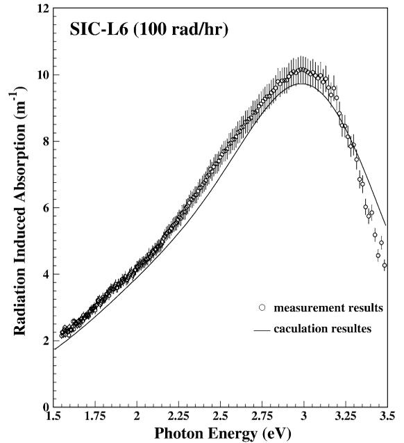
Fig. 8. The measured overall color center density as a function of energy in equilibrium under 100 rad/h is compared to model calculations for sample SIC-L6.
