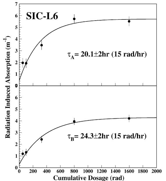
Fig. 4. The amplitude of the radiation-induced absorption centers is shown as a function of the cumulative dosage.
