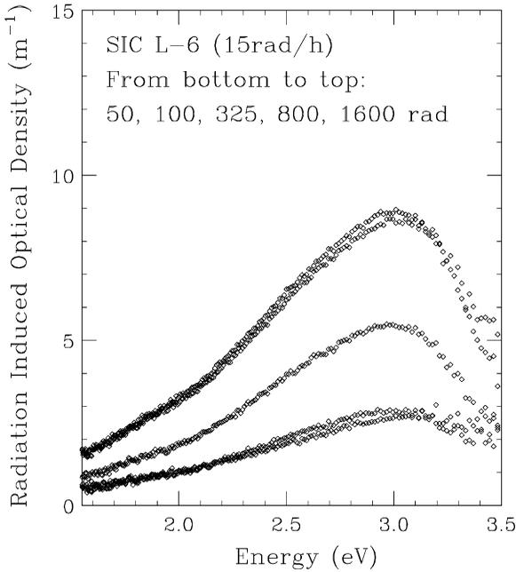
Fig. 2. Radiation-induced absorption is shown as a function of photon energy.
