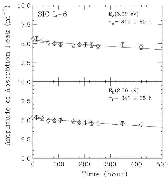
Fig. 6. The amplitudes of the absorption bands is shown as a function of recovery time.
