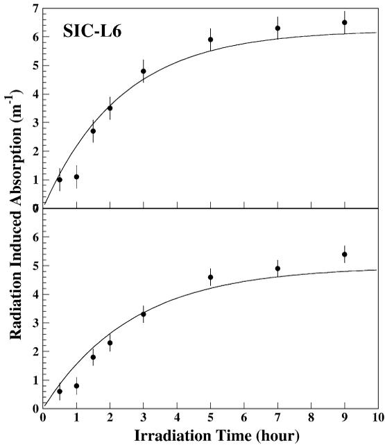
Fig. 7. The experimental data of the amplitudes of color centers A and B as a function of time under irradiation of 100 rad/h is compared to calculation by using kinetic model for SIC-L6.
