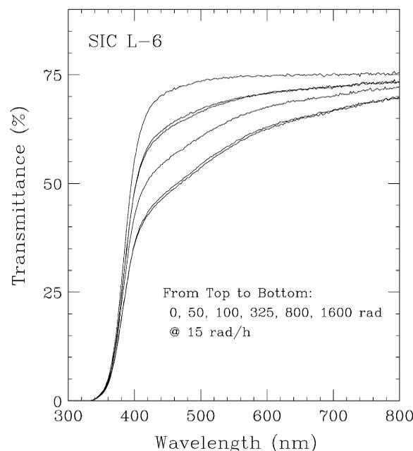
Fig. 1. The transmittance before and after irradiation is shown as a function of the wavelength.
