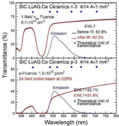
Fig. 2. Transmittance spectra for the LuAG ceramic samples n-3 (top) and p-3 (bottom) before and after a 1 MeV equivalent neutron fluence of  $6.7 \times 10^{15} \text{ n}_{\text{eq}}/\text{cm}^2$  at LANSCE and a proton fluence of  $1.2 \times 10^{15} \text{ p}/\text{cm}^2$  at CERN, respectively.
