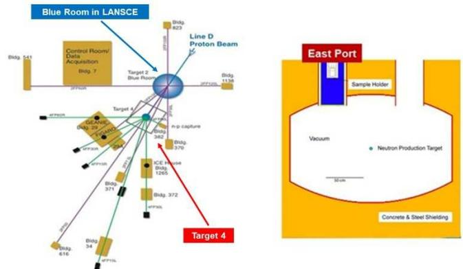
Fig. 1. The proton and neutron irradiation experiment sites in the blue room and the East Port of the Target 4 area of LANSCE (Left), and the sample location in the East Port (Right).
