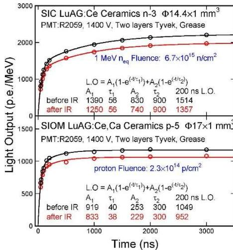
Fig. 3. Light output is shown as a function of integration time for LuAG ceramic samples n-3 (top) before and after a 1 MeV equivalent neutron fluence of  $6.7 \times 10^{15} \text{ n}_{\text{eq}}/\text{cm}^2$  and p-5 (bottom) before and after a proton fluence of  $2.3 \times 10^{14} \text{ p}/\text{cm}^2$  at LANSCE.
