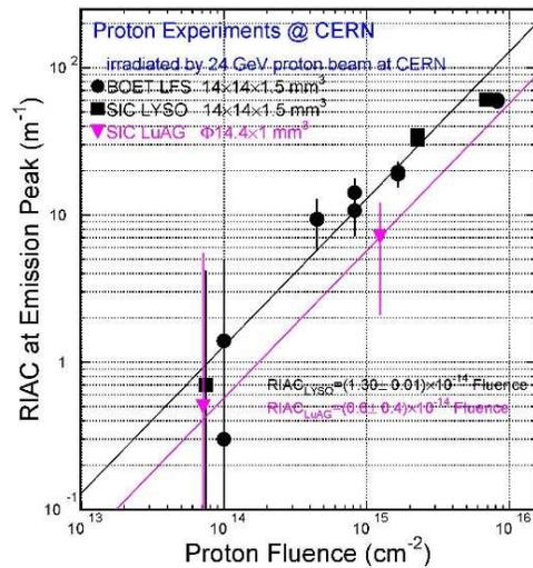
Fig. 5. RIAC as a function of proton fluence for the BOET LFS, SIC LYSO crystal and SIC LuAG ceramic samples irradiated at CERN.
