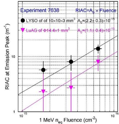
Fig. 4. RIAC as a function of 1 MeV equivalent neutron fluence for LYSO crystals and LuAG ceramics irradiated in the East Port of LANSCE.
