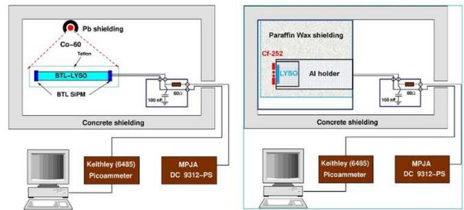
Fig. 1. A schematic showing setups used to measure photocurrent induced by Co-60  $\gamma$ -rays (left) and Cf-252 neutrons (right) in LYSO+SiPM packages.
