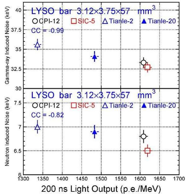
Fig. 4. Correlation between RIN: $\gamma$  (top) and RIN:n (bottom) vs. LO in 200 ns gate for four LYSO+SiPM packages.
