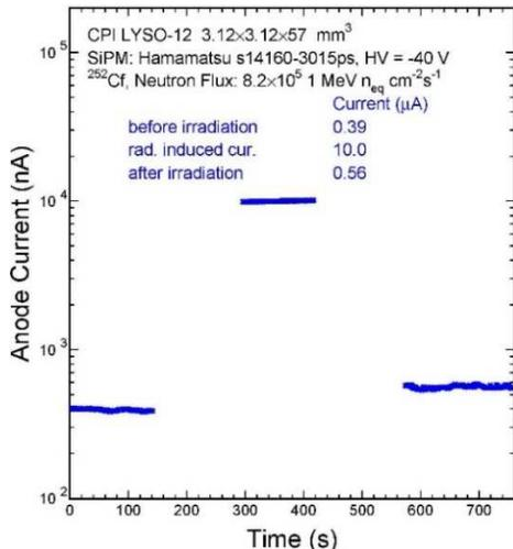
Fig. 3. Histories of photocurrent measured for the CPI LYSO+SiPM package under Cf-252 irradiation.
