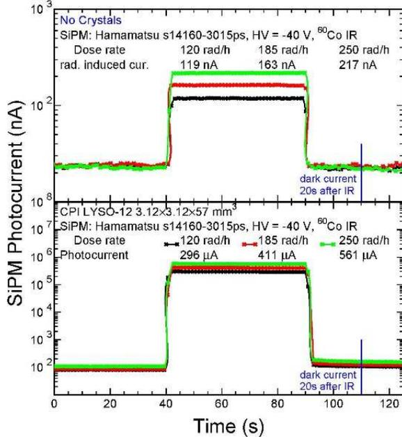
Fig. 2. Histories of photocurrent measured for the Hamamatsu SiPM (top) and the CPI LYSO+SiPM packages (bottom) under Co-60 irradiation.
