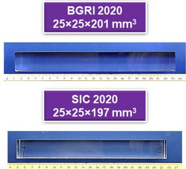
Fig. 1. Two BaF<sub>2</sub>:Y crystals grown by BGRI with a dimension of 25×25×201 mm<sup>3</sup> (top) and SIC with a dimension of 25×25×197 mm<sup>3</sup> (bottom) for the Mu2e-II experiment.
