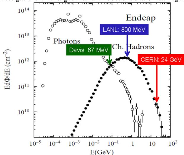
Fig. 1. Energy spectra of photons and charged hadrons expected at the HL-LHC calculated by FLUKA simulation. [1].
