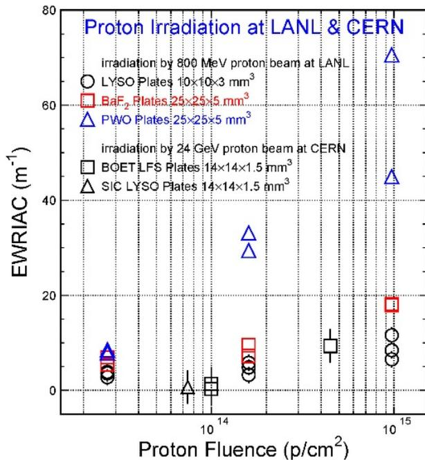
Fig. 3. EWRIAC values are shown as a function of proton fluence for LYSO, BaF<sub>2</sub> and PWO samples.
