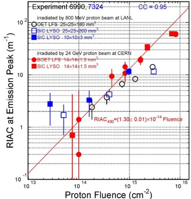
Fig. 5. The RIAC values at emission peak are shown as a function of proton fluence for LYSO/LFS crystals with various dimensions and vendors.
