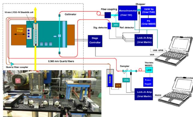
Fig. 2. A schematic showing the experimental setup used to measure crystal's transmittance spectra *in situ* during the experiment 7324. The inset photo shows the eight samples on the linear stage.
