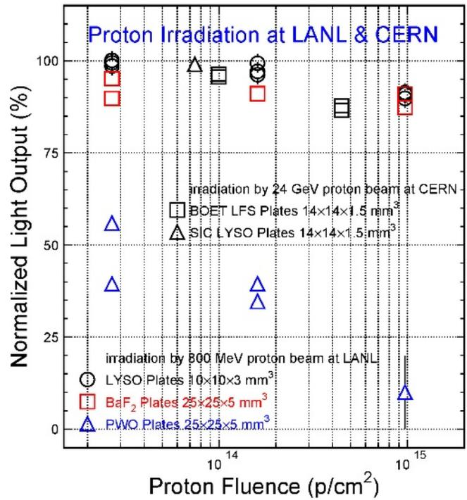
Fig. 4. Normalized light output is shown as a function of the proton fluence for LYSO, BaF<sub>2</sub> and PWO samples.
