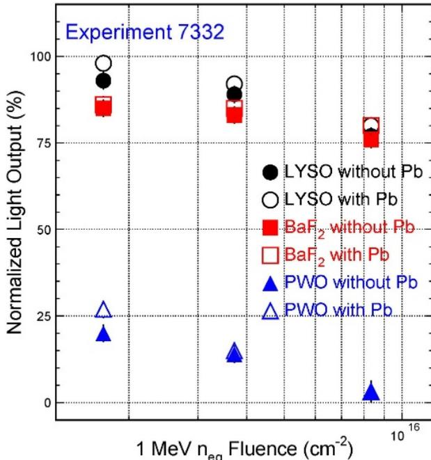
Fig. 3. Normalized LO is shown as a function of 1 MeV equivalent neutron fluence for LYSO, BaF<sub>2</sub> and PWO plates.
