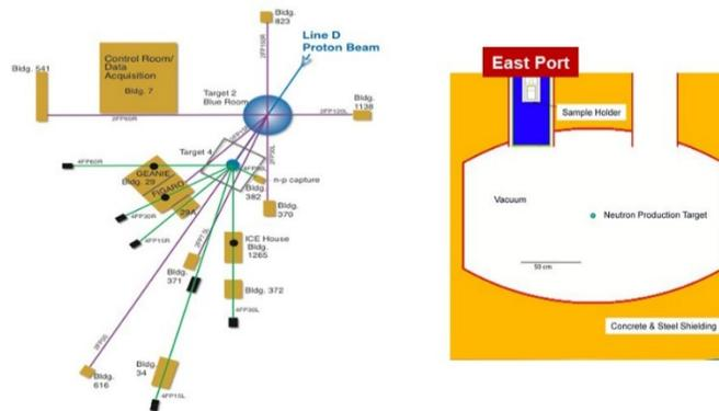
Fig. 1. Two schematics showing the neutron irradiation experiment site in the Target-4 area of LANSCE (Left), and the sample location at the East Port (Right).
