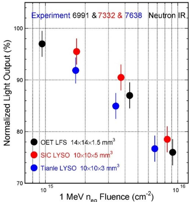
Fig. 5. Normalized LO is shown as a function of 1 MeV equivalent neutron fluence for LYSO plates used in three experiments from three vendors.
