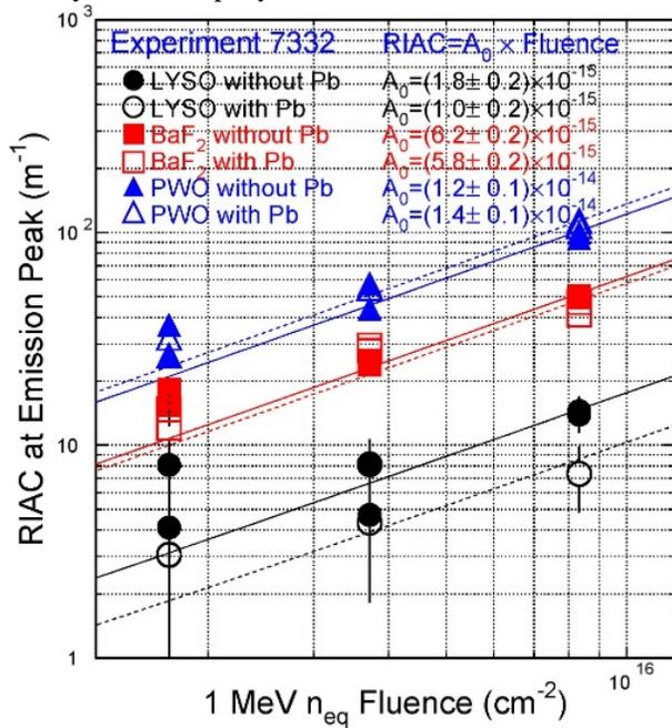
Fig. 2. RIAC values are shown as a function of 1 MeV equivalent neutron fluence for LYSO, BaF<sub>2</sub> and PWO plates.
