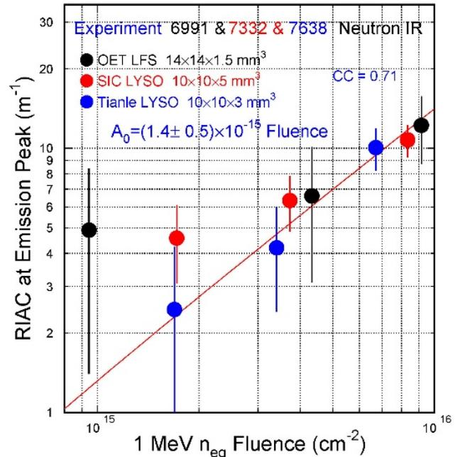
Fig. 4. RIAC values are shown as a function of 1 MeV equivalent neutron fluence for LYSO plates used in three experiments from three vendors.
