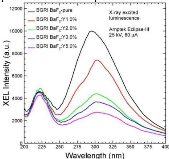
Fig. 1. X-ray excited emission spectra of BaF<sub>2</sub> non-doped and with yttrium doping of 1, 2.0, 3.0 and 5.0 at.%.
