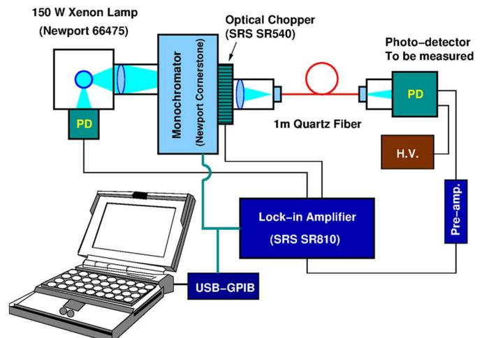
Fig. 2. A setup used to measure QE/PDE as a function of wavelength.
