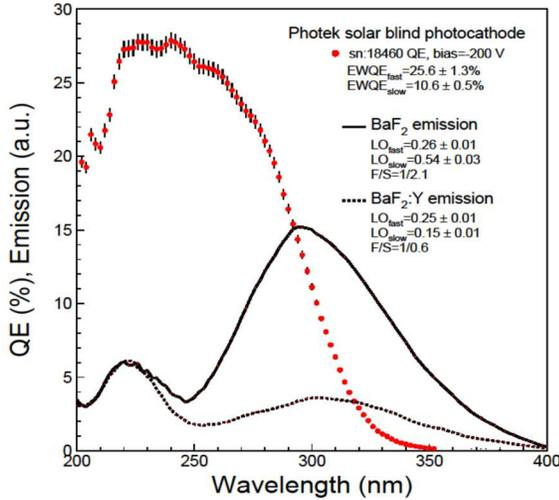
Fig. 4. The measured QE (200-400 nm) of Photek solar blind photocathode and the X-ray excited emission spectra of BaF<sub>2</sub> and BaF<sub>2</sub>:Y.
