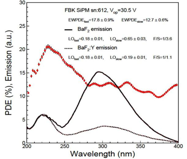
Fig. 5. The measured PDE (200-400 nm) of a FBK SiPM with type-I UV filter and the X-ray excited emission spectra of BaF<sub>2</sub> and BaF<sub>2</sub>:Y.
