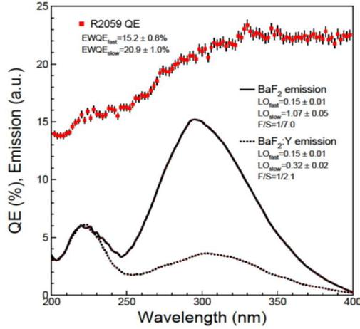
Fig. 3. The measured QE (200-400 nm) of a Hamamatsu R2059 PMT and the X-ray excited emission spectra of BaF<sub>2</sub> and BaF<sub>2</sub>:Y.
